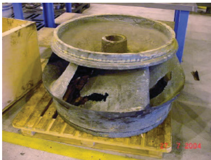
Figure 6 Severe corrosion of an NAB pump impeller due to sulphide pollution.
