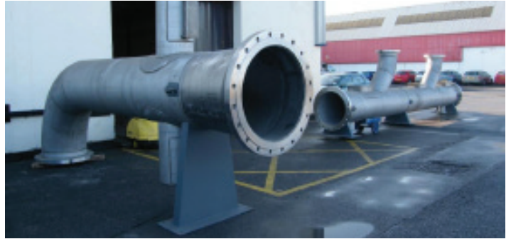
Two sections of a superduplex stainless steel manifold for the seawater cooling system of a large alumina plant.
