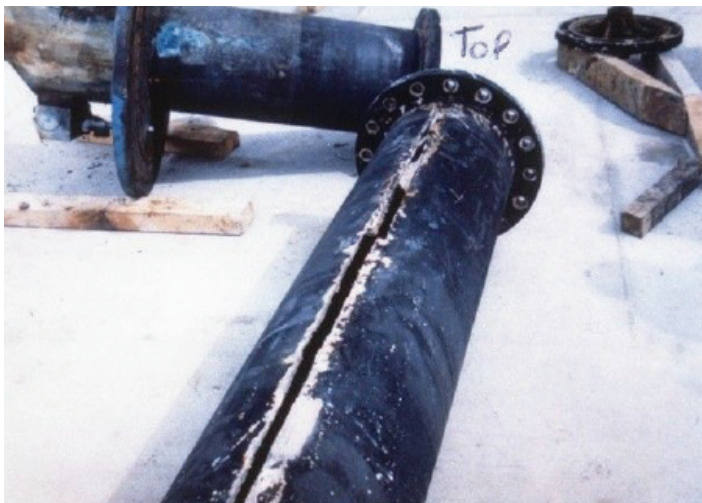
Figure 1 Corrosion of the beta phase in an NAB seam welded pipe that had not been post weld heat treated.
